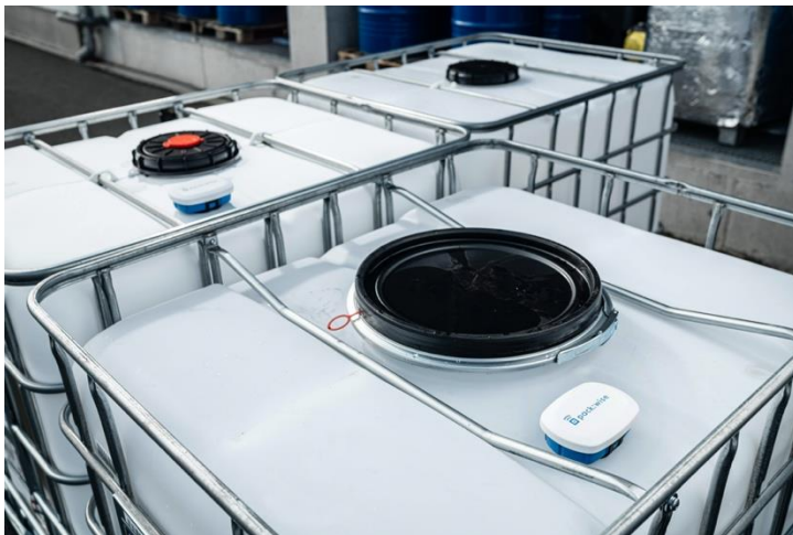
Photo 3: Packwise Smart Cap in use on intermediate bulk containers
